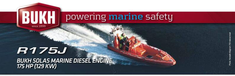
The BUKH R-Series Solenoid Common Rail Direct injection System(CRDi) delivers 175 hp and 440 Nm of torque from the 2.2 liter In-line 4 CRDI engine.
